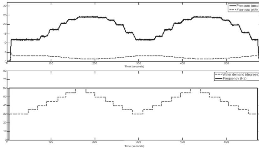
**Figura 4.** System operating without the action of the controller.
