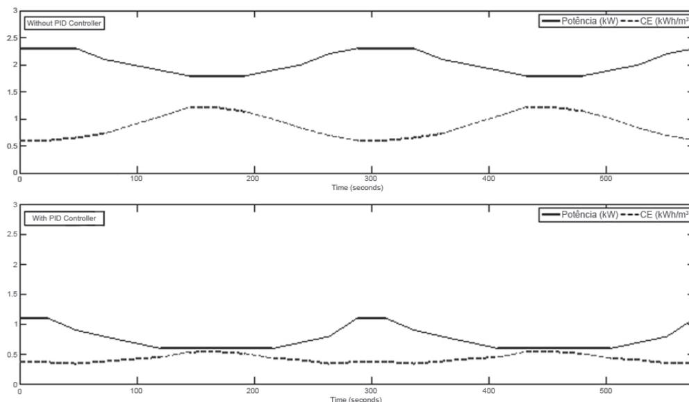
**Figura 6.** Power value and SEC comparison by the system with and without the PID controller.
