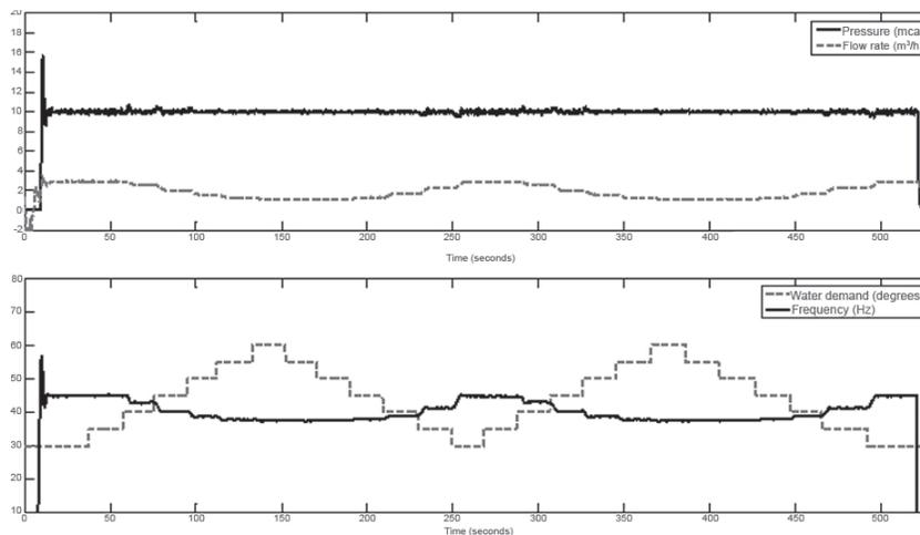
**Figura 5.** System operating with the action of the PID controller.
