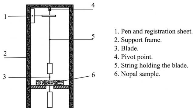
Figure 1. Pendulum for determination of cutting energy.
