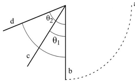
Figure 2. Pendulum diagram used to determine the cutting energy.
