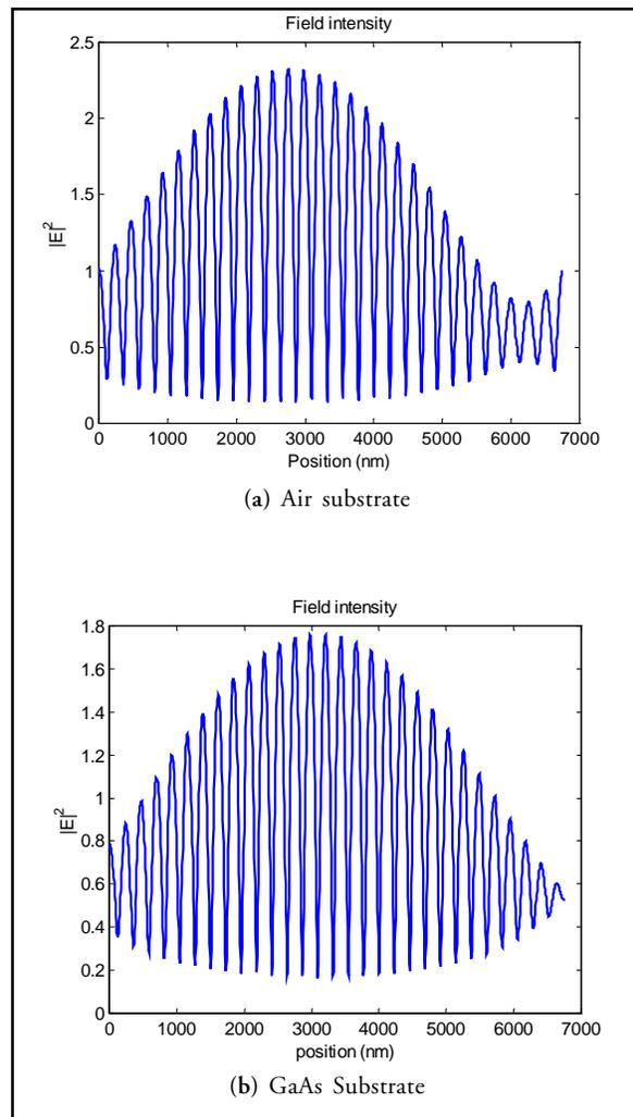
Figure 3. Envelope of the field for a 30 period multi-layer stack. (a) Has an air substrate and (b) has a GaAs substrate. The field is shown for the first transmission maximum, which occurs at the wavelength,  $\lambda=1608.7 \text{ nm}$  (a), and  $\lambda=1606.2 \text{ nm}$  (b). Note the vertical axis should be  $|E|$  and not its square.
