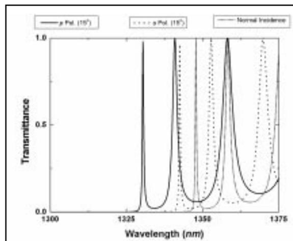
Figure 9. Transmission spectra for normal incidence and 15 degree angle of incidence. The p- and s-polarizations have different shifts of their band-edge resonance peaks, but the resonance width is nearly the same.
