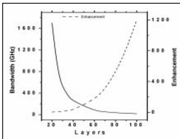
Figura 8. Down-conversion signal enhancement and bandwidth versus the number of layer pairs for GaAs/Al<sub>2</sub>O<sub>3</sub> PBGs. The parameters are the same as in Fig. 5.
