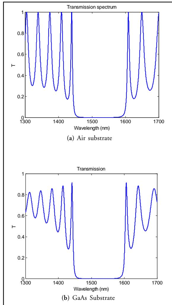
Figure 2. Transmission spectrum for 30 periods GaAs/AlAs. Air substrate (a) and infinite GaAs substrate (b).
