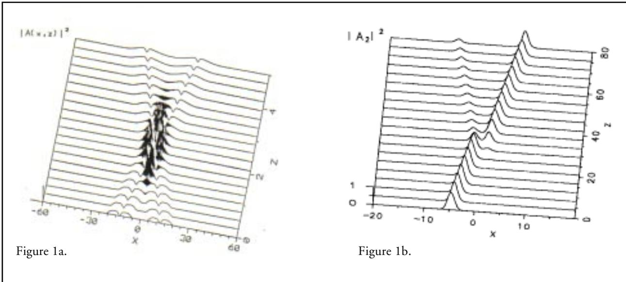
**Figure 1a, 1b.** Numerical simulation demonstrating the ability of crossing of two optical waveguides based on ideal dark spatial solitons to act as an asymmetric optical Y-junction. In (a) we show the soliton collision and in (b) the trajectory followed by the guided beam. The ideal solitons are characterized by the parameter  $\lambda = 0.12$ , and in the eq.(1) we used:  $r_k r_n = 1$  and  $\beta = 1.8$ .
