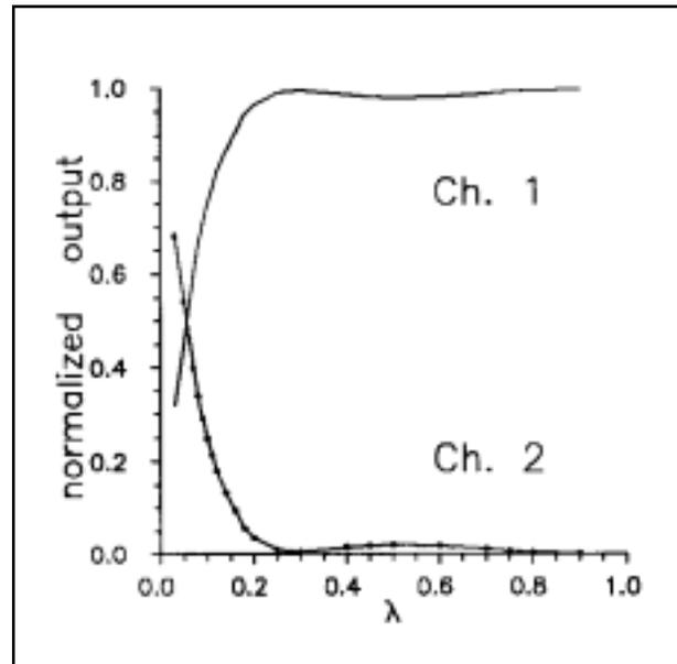
**Figure 2.** The normalized output energy of the probe beam in each optical channel after the collision of two ideal dark solitons as a function of the soliton parameter  $\lambda$ . For relative large collision angles, the probe beam basically follows the original waveguide (1), but for small angles the energy of the probe beam guided by second channel progressively increases. Here  $r_k r_n = 1$  and  $b = 1.8$ .
