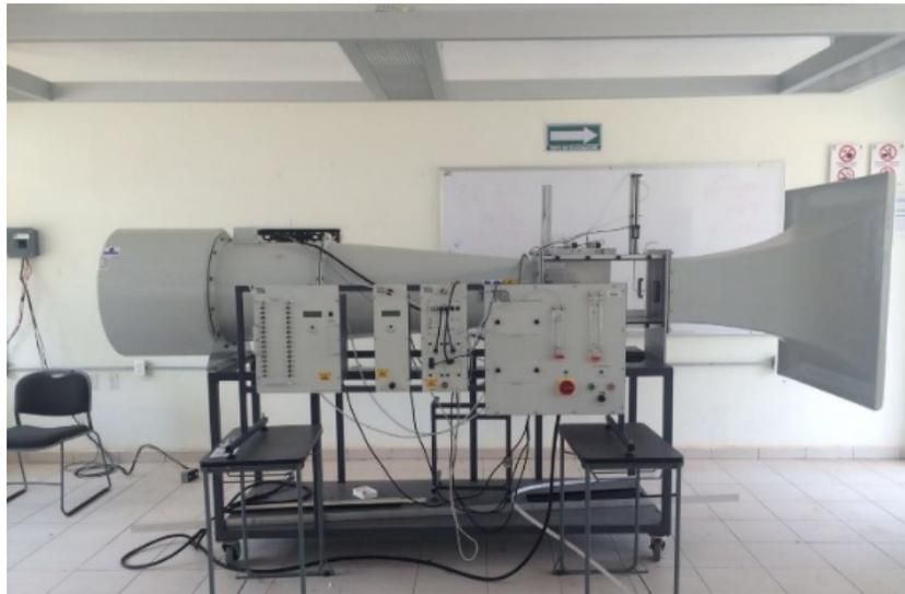
Figure 6. TecQuipment AF100 subsonic wind tunnel used in the aerodynamic test of the 3D UAV model.
