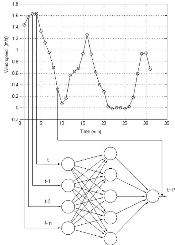
Figure 11 . Artificial Neuronal Network Input and output.
