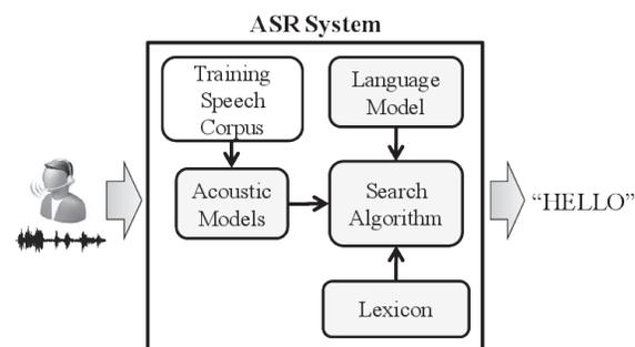
Figure 4 . Functional elements of an ASR system.
