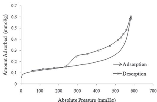
Figure 2.  $\text{N}_2$  adsorption-desorption isotherm of tezontle for average 425  $\mu\text{m}$  size fraction.
