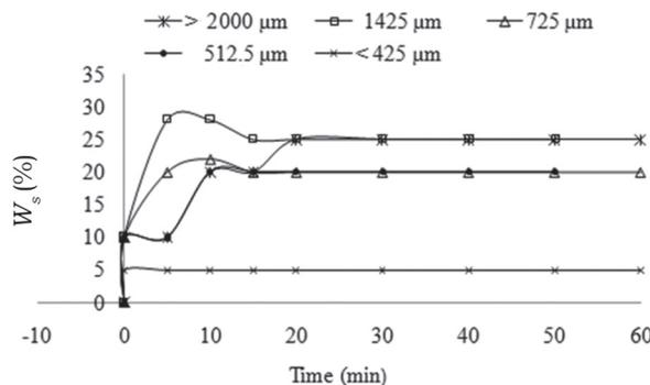
Figure 1. Swelling kinetics of different mean-particle-diameter fractions of red tezontle.
