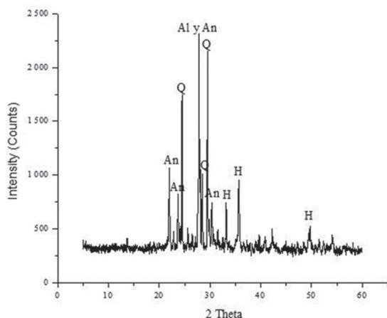
**Figure 3.** X-rays diffractogram of tezontle. Peaks from: Quartz (Q), anorthite (An), albite (Al) and hematite (H).
