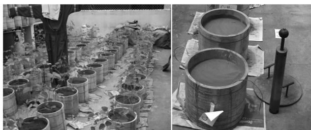
Figure 1. Experiment view of the sixty-four treatments. Cylinders, Proctor hammer, Proctor bump support and moisture meters used in the study. Source: Authors own elaboration.
