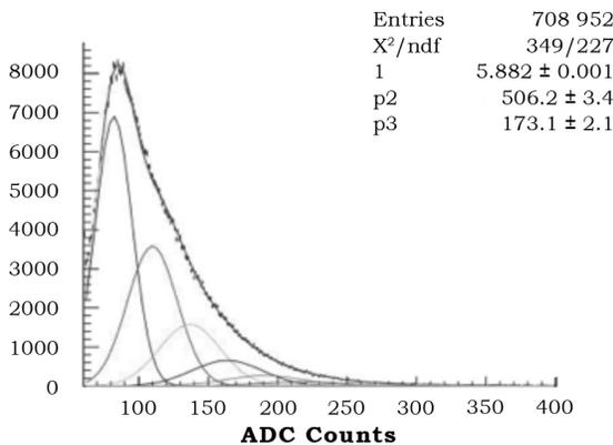
**Figure 4.** Top panel: Fit to the one  $p.e.$  ADC distribution using a tiny hole: the histogram shows the data, the first gaussian curve from shows the one  $p.e.$  distribution, and the second and third gaussian curves from the left show the two and three  $p.e.$  distributions. The on top of the histogram bars is the sum of these distributions. Bottom panel: The ADC distribution and the several  $p.e.$  fits for a mask with two holes of 1.19 mm of radius. Source: Author's own elaboration.
