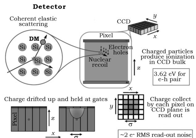
Figure 2. The DAMIC CCD operation.
