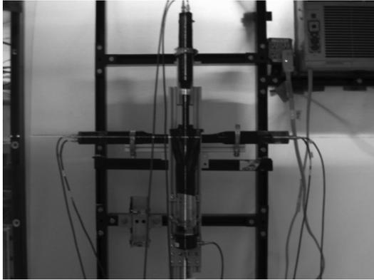
**Figure 3.** The two scintillator bar experimental setup at the Fermilab Test Beam Facility. Laser light is used to align the array with the proton beam direction. Source: Author's own elaboration.
