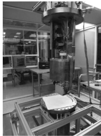
Figure 1. The DAMIC CCD array (top) and the vacuum vessel with vacuum and temperature controllers (bottom).
